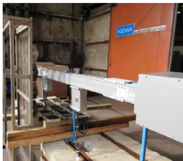
Fig 1: IEC 61641 Test Setup
